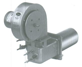
The Eclipse Minimatic burner is a compact packaged gas burner designed for fixed air operation at firing rates up to 400,000 Btu/hr. It is used in process air heating applications, such as ovens and dryers. The 40 MMB-FA Model features an adjustable air inlet damper for setting air flow in proportion with the desired burner firing rate.
